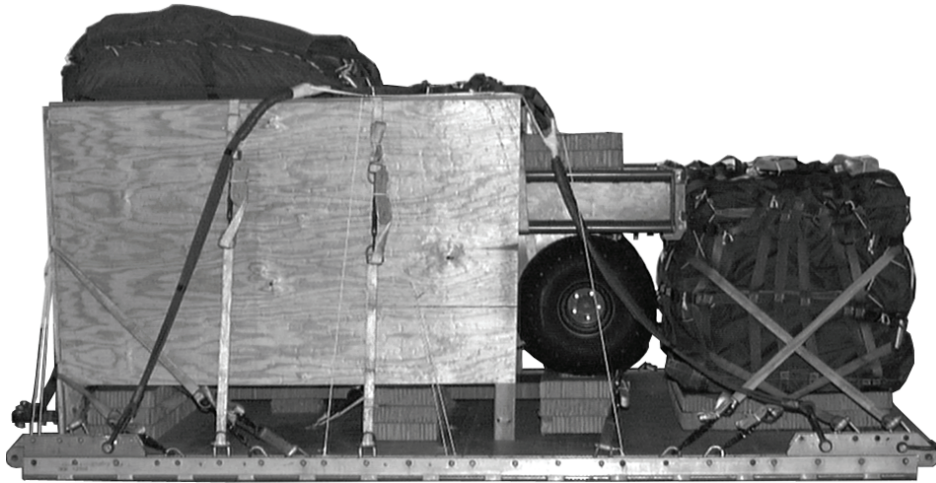
One Military Utility Vehicle (M-Gator) and an A-22 Cargo Bag on a 12-Foot Platform
